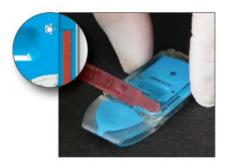
Insert the syringe tip into the sample well and slowly twist and push the plunger until the sample reaches the fill mark.
